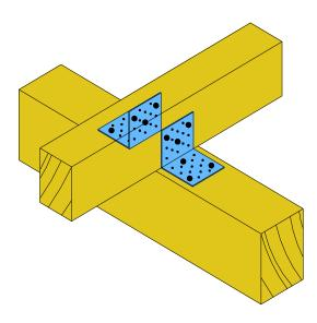
Figure B.2 Typical installation of BREKAR angle brackets
